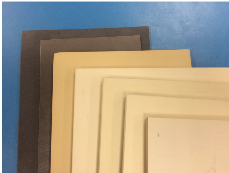
Figure 3.10 Rogers microwave materials with metal backplane and properties listed in Table 3.4. From top left to bottom right: RT/d5870, RT/d5880, TMM3, TMM4, TMM6, TMM10 and TMM10i.
